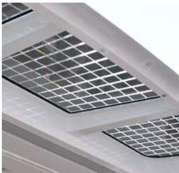
Its space has been designed to optimize its photovoltaic panel surface. The 8.2 kW of solar panels on board the boat represent much more than just energy sources. They embody our commitment to ecological and sustainable navigation. Thanks to this solar installation and lithium batteries, the boat is self-sufficient in electricity.
