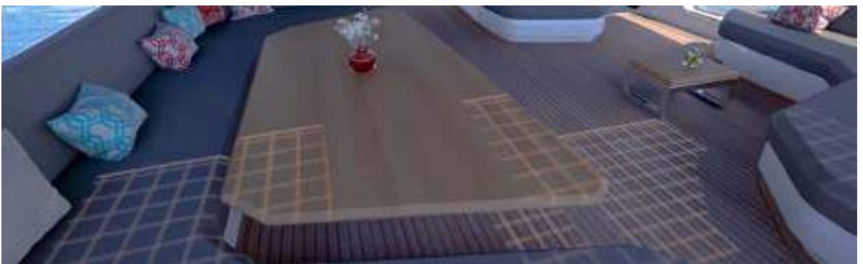
The power of these solar panels has not been left to chance: the surface has been carefully studied to optimize the energy yield, reaching 8.2 KW, to supply the boat's hotel load with energy, including the air conditioning in eco mode in the cabins.
